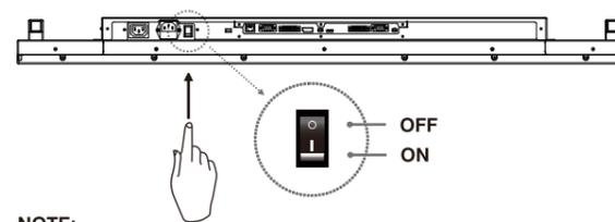
**NOTE:** The remote control only works when the mains switch is in the ON position.
